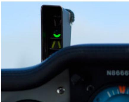
*As the airplane slows on approach (top) it reaches its optimum AOA (above), signified by the green circle. By maintaining optimum AOA on approach, pilots avoid going too fast or too slow.*
